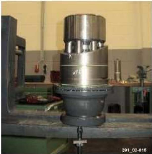
**MOTOR HIDRAULICO DE UNA TRANSMISION HIDROSTATICA, CON SU CONJUNTO DE FRENO.**
